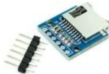
SK2 - Micro SD card module
